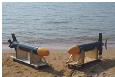
图 5 SPC-III 仿生水下航行器(右)与无人水下航行器(左)对比 Fig.5 Comparison of SPC-III biorobotic AUV (the right one) and an AUV (the left one)
