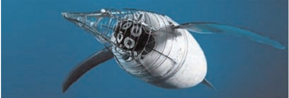
图 9 Festo 研发的仿生企鹅 AquaPenguin 样机 Fig.9 The bionic AUV named AquaPenguin developed by Festo
