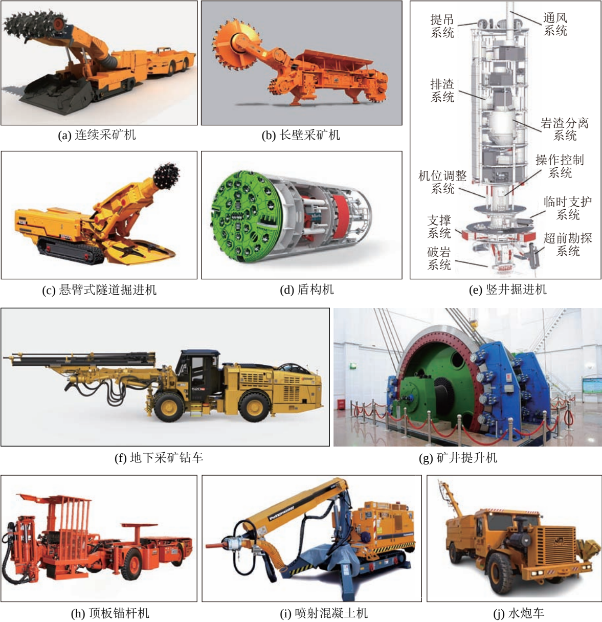
图 14 地面深层开采作业设备 Fig.14 Equipments for deep surface mining operations
