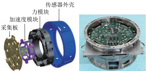
图 1 12 维传感器系统原理图及实物照片 Fig.1 System diagram and photo of 12-DOF sensor
