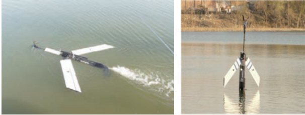
图6 北京航空航天大学“鳀鸟”潜水无人机 Fig.6 Submersible UAV “Gannet” developed by Beihang University
