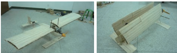
图7 南昌航空大学的潜水无人机样机 Fig.7 Submersible UAV prototype developed by Nanchang Hangkong University
